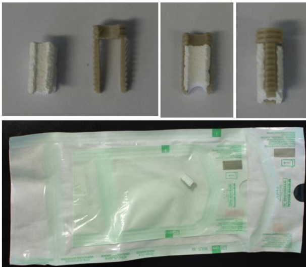
Figure 6.2 The photos of TCP insert, PEEK anchor housing, assembled anchor, and sterilized anchor.
