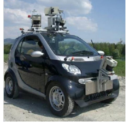
Fig. 2. Our autonomous Smart car platform. There are three fixed laser range finders mounted on the front of the vehicle and on the sides of the roof, and two spinning laser range finders mounted together on the center of the roof.
