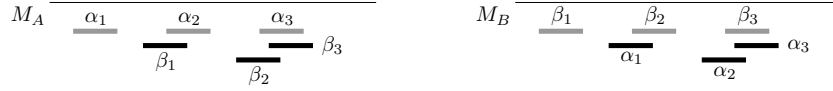
Figure 1: Instance where A^3 returns exactly 2/3 \cdot |O| jobs: O contains all jobs \alpha_i and \beta_i for i = 1, 2, 3 (in grey), but both A^2(M_A, M_B) and A^2(M_B, M_A) schedule only the jobs \alpha_1, \alpha_2, \beta_1, \beta_2 .
