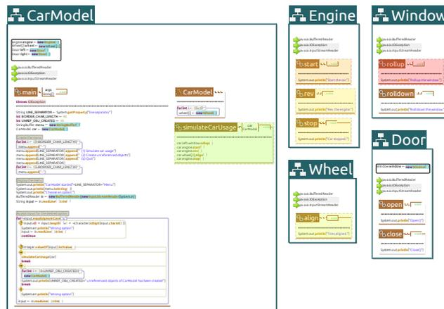
Figure 8.2: A heatmap overlaid on top of Envision's usual code presentation. The heatmap is visualized as a set of translucent overlays on top of methods; each overlay has a color in the spectrum between red and green, indicating how often a method was executed.
