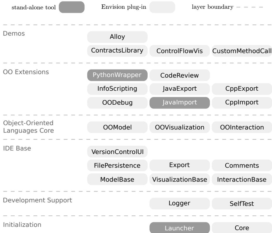
**Figure 4.1: The layers of Envision’s architecture including all current plug-ins and stand-alone tools.**
