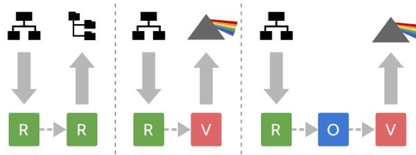
**Figure 8.5:** The three common types of queries: (R) resource-access, (V) visualization, and (O) operator. On the left a resource-access query extracts information from an AST and forwards it to another query, which writes it to a file. In the middle, this information is being visualized instead of written to file. On the right, an additional filter is inserted to refine what information is displayed.
