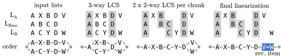
**Figure 7.7: Computing a total order for the elements of a merged list. Stable chunks have a light-gray background. At the end,  $V$  and  $W$  are linearized and added to a review item. In the merged list,  $B$  and  $C$  will be removed to reflect changes from revisions.**
