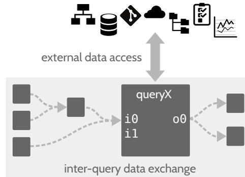
**Figure 8.4: A query network with seven interconnected queries. *queryX* is shown in detail. It has two inputs (*i0*, which is the union of two outputs from other queries and *i1*, which is unused here), and one output (*o0*, which is duplicated).**
