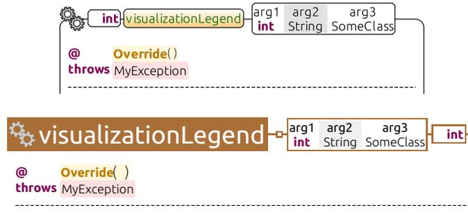
**Figure 5.7:** A method (⚙️) signature using an early (top) and the current (bottom) Envision visual design.
