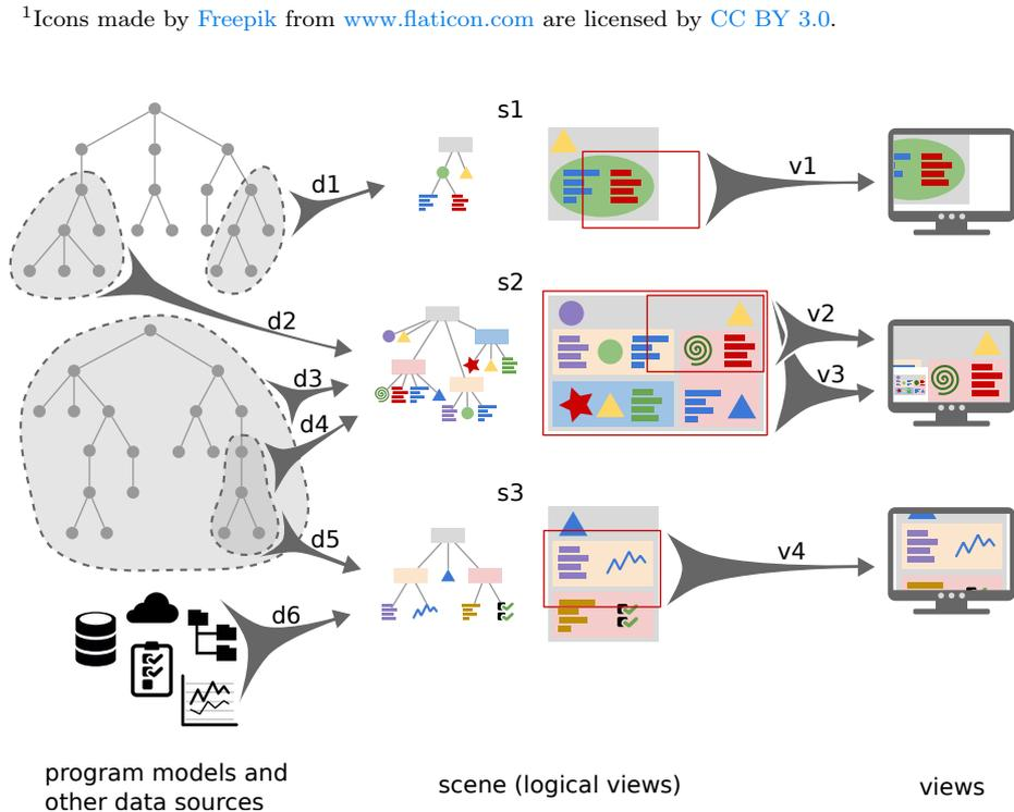
**Figure 5.2: An illustration of composing and rendering visualizations in Envision. There are six (d)ata sources; three (s)cenés; and four (v)iews.<sup>1</sup>**
