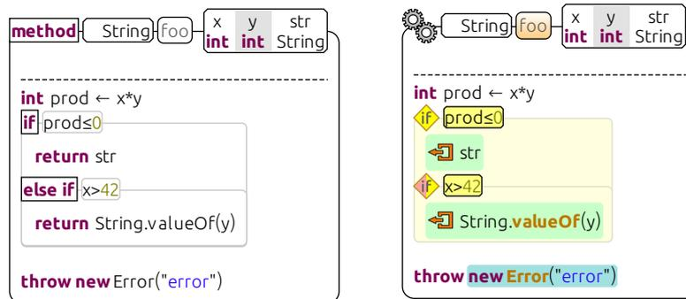
Figure 4.2: Two alternative visual styles for displaying methods in Envision.
