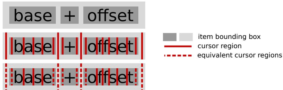
**Figure 6.3:** Four visual items representing the expression `base+offset` wrapped in a container. Top: the items' bounding boxes; middle: cursor regions without equivalent regions; bottom: cursor regions with equivalent regions.
