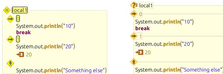
Figure 5.11: A switch-statement (🔍) with two specified cases (➡) and a default case (⬇) in an early (left) and the current (right) Envision visual design.
