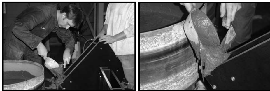
Figure 4.6: Casting of the 'U-shaped' specimen: the mould is given an inclination to prevent "free fall" of the concrete along the "A"-side
