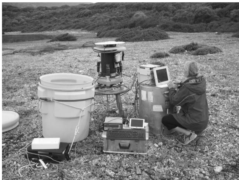
Figure 7.11: Preparation of an observation with DIADEM on the island of Kira Panagia. The ton served as shipping container for DIADEM. For the transportation by boat, the ton has been mounted at the stern (Fig. 7.13b). In order to perform differential GPS measurements, a GPS antenna is temporarily fixed on top of DIADEM. The antenna is removed when starting the DIADEM observations.
