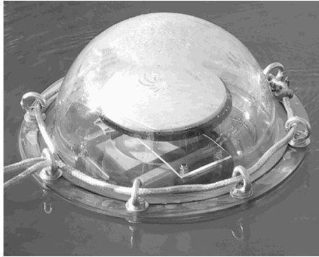
a) Waterproofed buoy equipped with GPS receiver, antenna and battery.
