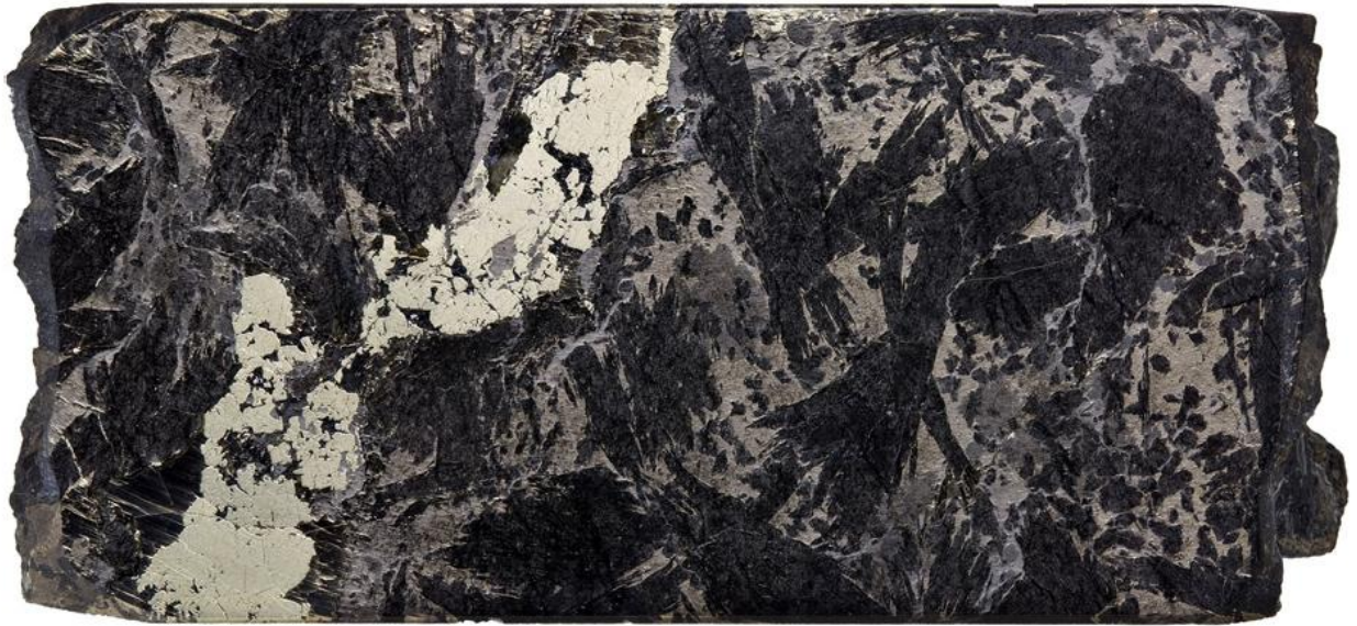
Fig 15-2-5. A black metacarbonate rock with abundant tremolite, sulphides and graphite. The black metacarbonate rocks occur as 0.5- to 3.0-m-thick intercalations in black schist. The width of the core section is 3 cm (Loukola-Ruskeeniemi and Lahtinen, 2013).
