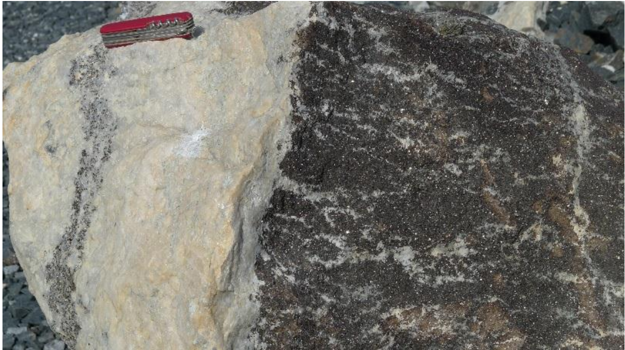
Fig. 15-1-10. Internal magmatic contact within the Siilinjärvi carbonate, showing earlier banded phlogopite carbonate (also called glimmerite if carbonate content is less than a few percent; right side of photo). This magmatic banding is truncated by later intrusion of weakly biotite-bearing but apatite-rich carbonatite composed of 60% cream-colored calcite and 30% pale green apatite. (photo: Ch. Heinrich).
