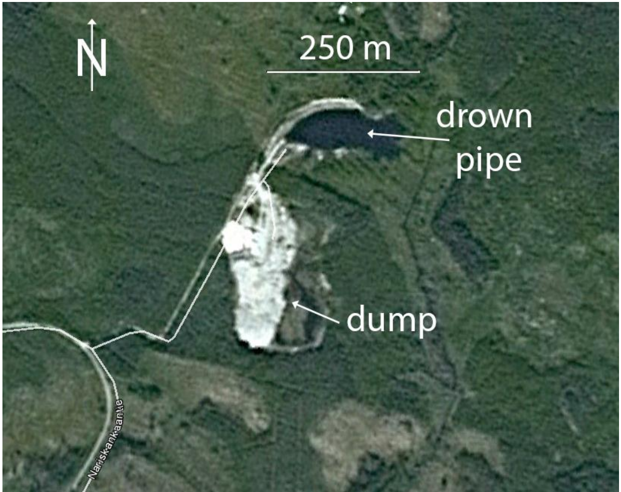
Fig 13-2-2. Google Earth™ image of Lathojoki test pitting. The actual pit is drown. Note the small size of the occurrence.
