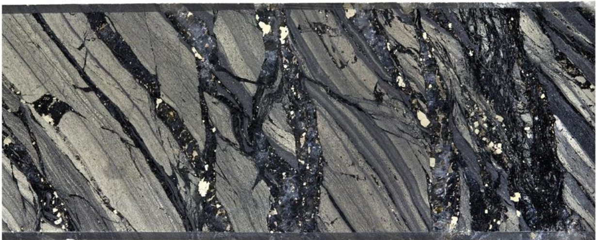
Fig 15-2-4. Synsedimentary/syndiagenetic laminae in black schist rich in graphite and spheroidal fine-grained pyrite. The lamination is cut by quartz-sulphide veins with coarse-grained pyrite. The width of the core section is 3 cm (Loukola-Ruskeeniemi and Lahtinen, 2013).
