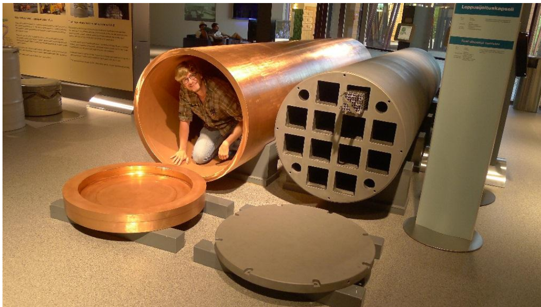
Fig. 26-1-5. Large Cu tubes (left) as used for longterm storage of fuel rods in steel casing (right), the power plant exhibition (photo: Ch. Heinrich).
