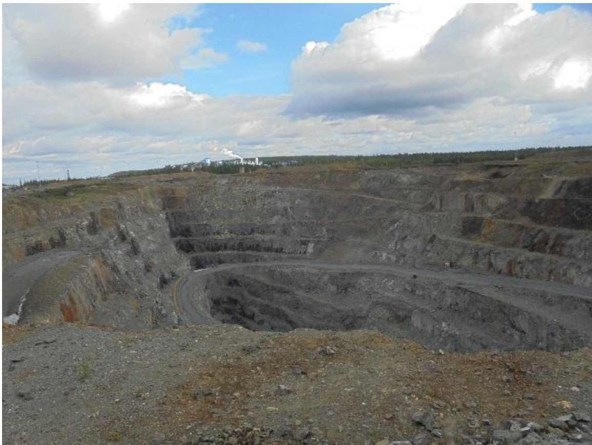
Fig. 18-1-12. Open-pit of Kittilä: Wedging out of the ore body on the opposite wall of the pit (photo: Ch. Bovier).
