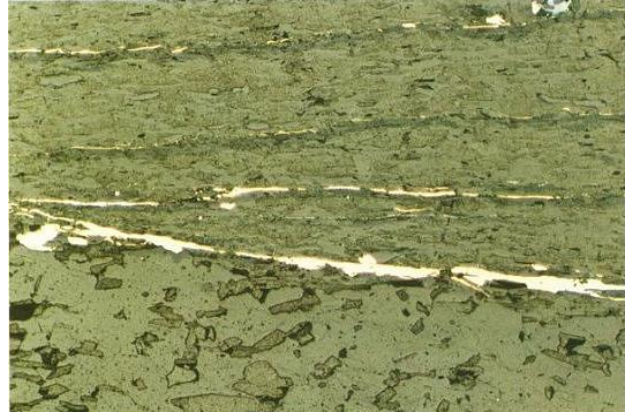
Fig. 16-2-5. Veinlets of gold, tellurides and Bi minerals in sericite-quartz rock (from Pankka, 1992).
