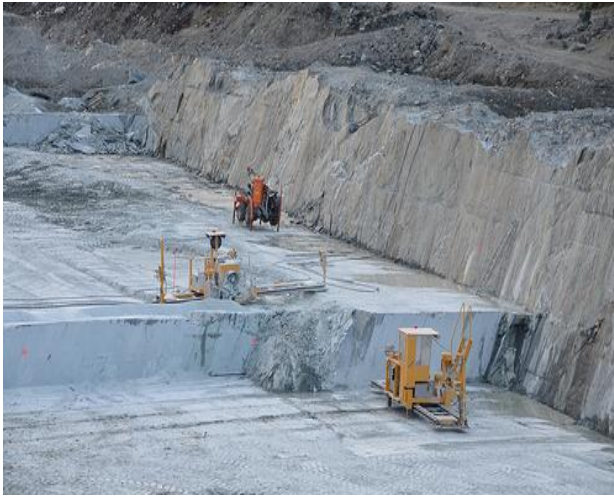
Fig. 13-1-2. Soapstone quarry and sawing machinery (www.flickr.com).
