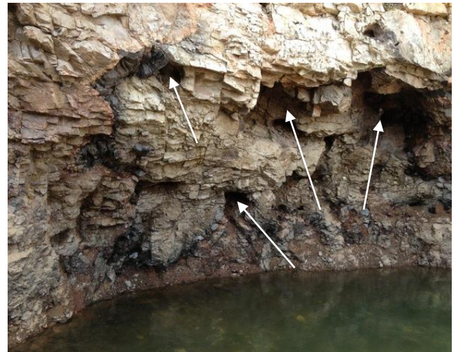
Fig. 12-1-12. Open pit exposure of the Luumäki pegmatite showing feldspar-rich pegmatite (left and near water line), the biotite rich transition zone with small workings where beryl was presumably extracted (arrows), and the inner quartz core. Photo by T. Rönkä.
