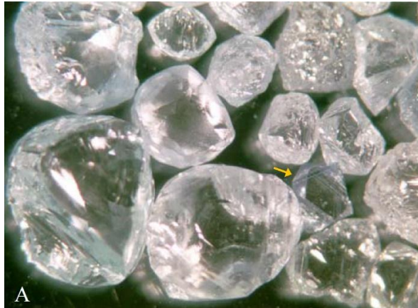
Fig 13-2-6. Lahtojoki diamonds (largest stone = 1ct). The diamonds appear clear but highly resorbed, sometimes with frosted surface (3 rd diamond from the left). Exception is a little octahedron (yellow arrow) with no apparent resorption features. Picture from O'Brien & Lehtonen (2008).
