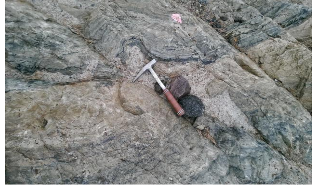
Fig. 16-2-9. Juomasuo test pit: Contact between altered metasediments and metavolcanic rocks (photo: D. Klimentyeva).
