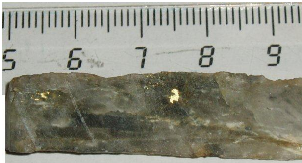
Fig. 25-3-2. Ania: visible gold in quartz vein, scale in cm, Kärkkäinen et al., 2006 (rom GTK website).
