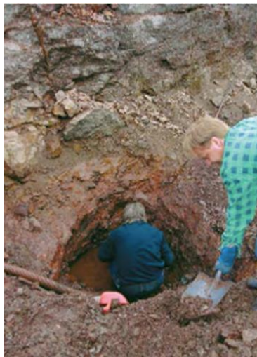
Fig. 12-1-11. The extraction of the beryl crystals has to be reduced to mining by hand to avoid any damage of the crystals. [3] Photo by P. Lyckberg.
