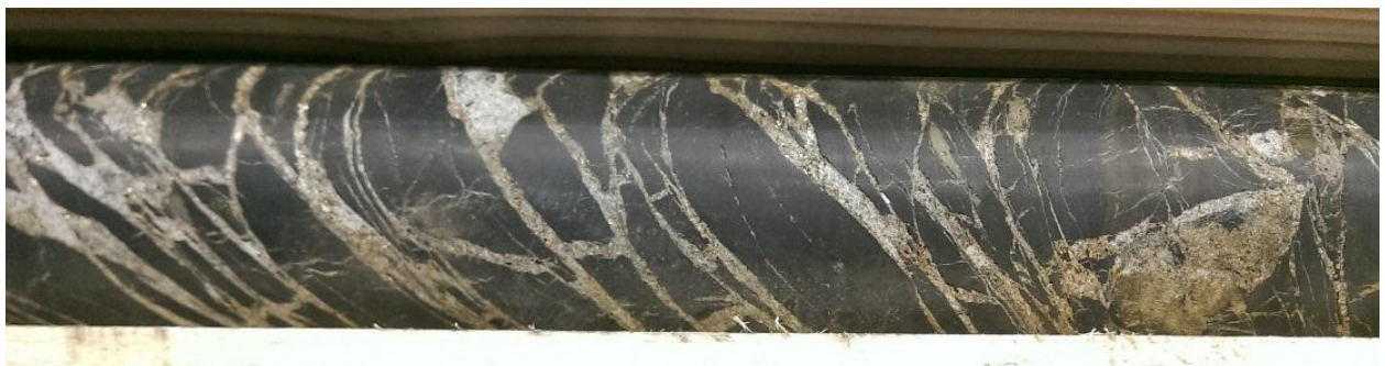
Fig. 14-2-9. Deformation and brecciation structures in drill core (photo: D. Klimentyeva).
