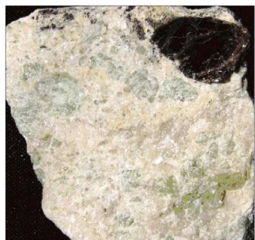
Fig. 15-1-6. Medium-grained calcite carbonatite with apatite (greenish) and one 3-cm-wide phlogopite book. From Lehtinen et al (2005).
