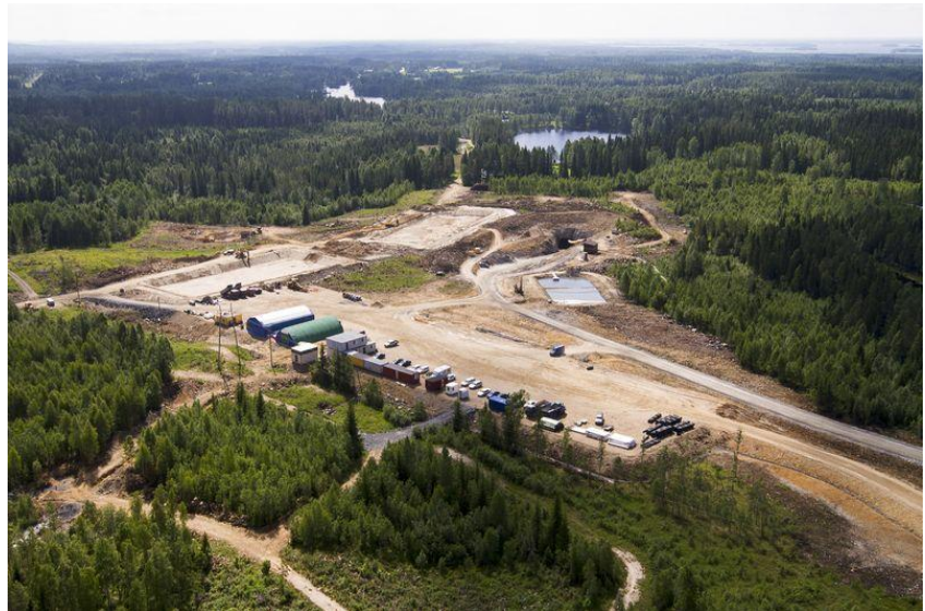
Fig 14-2-7. Kylylahti mine site with temporary offices, water storage ponds under construction and decline entrance. [2]
