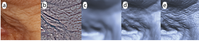
Figure 7: This figure demonstrates the effect of the mesoscopic-consistency term. The captured image (a) is filtered to extract the mesoscopic detail (b). In (c), the Poisson-reconstructed surface is shown. The refinement described in Section 3.2 already enhances the coarse geometry (d), but only the mesoscopic formulation is capable of reproducing the fine-scale details (e).
