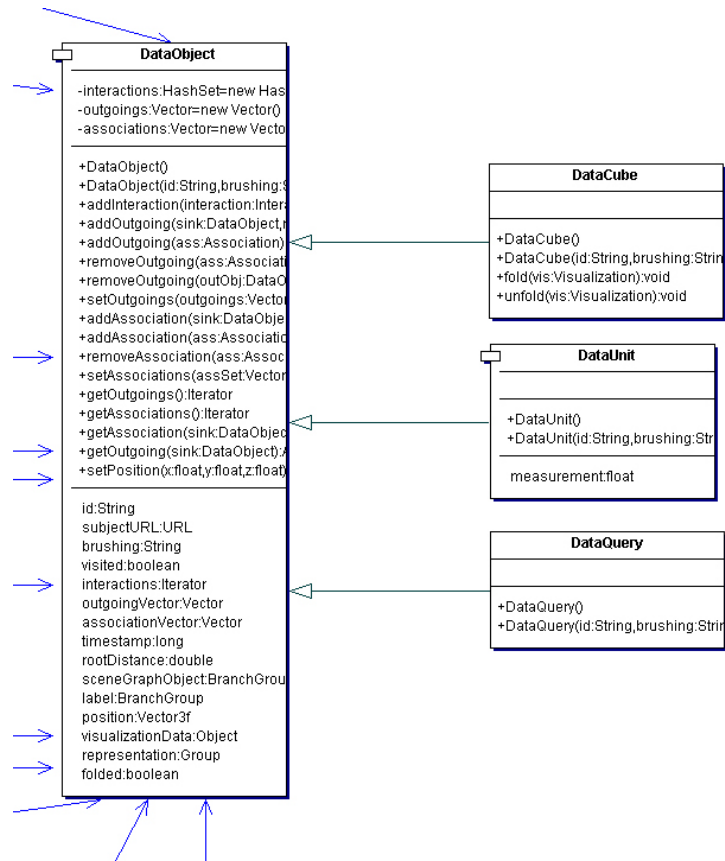
Figure 5.4: Part of the Class Diagram showing the Different Data Objects
